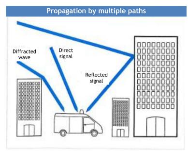
On reception (by our GONIO, for example), all these signals become combined as a set of multi-path components: the signal received is the sum of the principal signal and of all the reflected signals (from the ground, vegetation, water surfaces, buildings or other structures, etc.).
