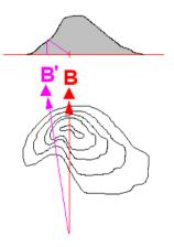
The figure opposite shows a transmitter B (in red) masked by a high hill. The signal from the transmitter is naturally considerably attenuated but remains audible, as the waves circumvent the obstacle. In this particular case, the shape of the obstacle and the position of the transmitter cause the signal to appear to come from the left (represented by B' in violet).
